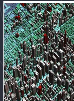
3D LiDAR-derived image of midtown Manhattan. This image shows change detection of new buildings highlighted in red, using 2010 and 2014 nDSM LiDAR data. Detected changes were used in a Department of Finance pilot program to identify property assessment changes.
